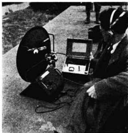
The 2,350 Mc/s. station operated by G3CBN/P at High Salvington, Sussex, when a distance of 13 miles was covered. Using the same gear the record now stands at nearly twice this distance.
